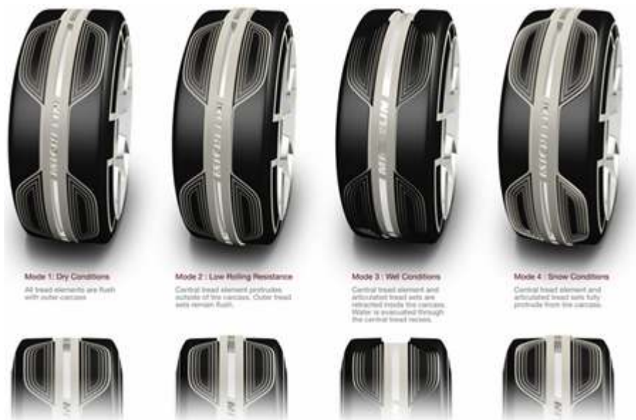
Abb. 167 Adaptive Reifen Quelle http://www.autoblog.com/2006/04/26/mighty-morphin-tire-technology-on-mazda-rx-9/
